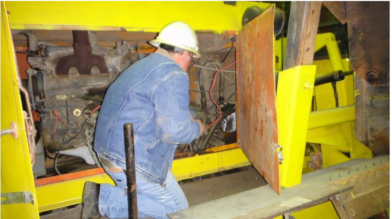
Mike H. takes on the ballast regulator's leaky hydraulic filter
