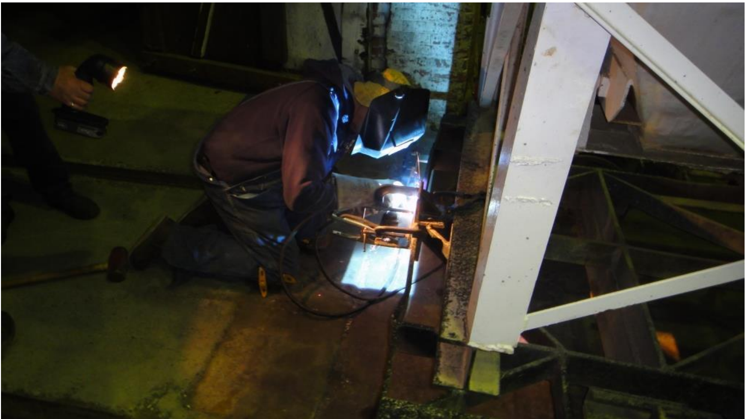
Cliff welds the draw-bar coupler back onto the ballast hopper car
