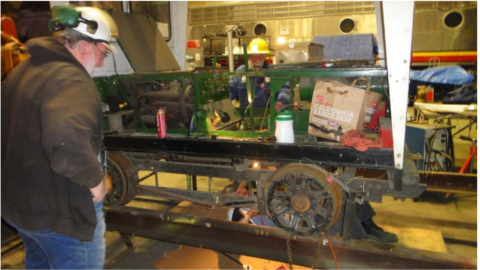
Frank, Pat, and Fred (under the machine) take apart the A-4 motorcar's transmission to replace the clutch
