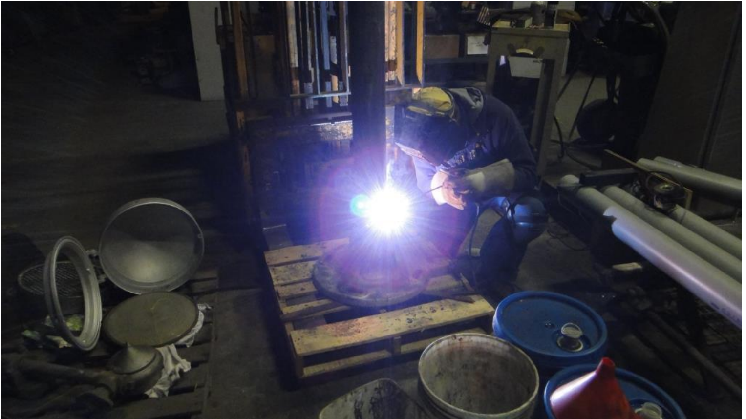
Cliff welds the signal post to the stand
